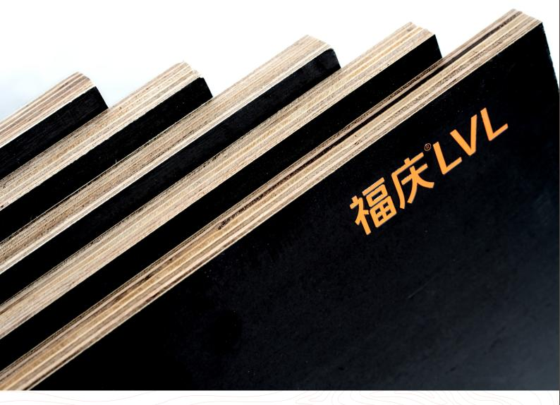
Fuging F17 Formply is made with high-quality hardwood veneers bonded with waterproof phenolic resin glue, ensuring superior strength and moisture resistance. Its smooth film coating provides a non-stick surface for concrete, allowing for easy removal and multiple reuses.
