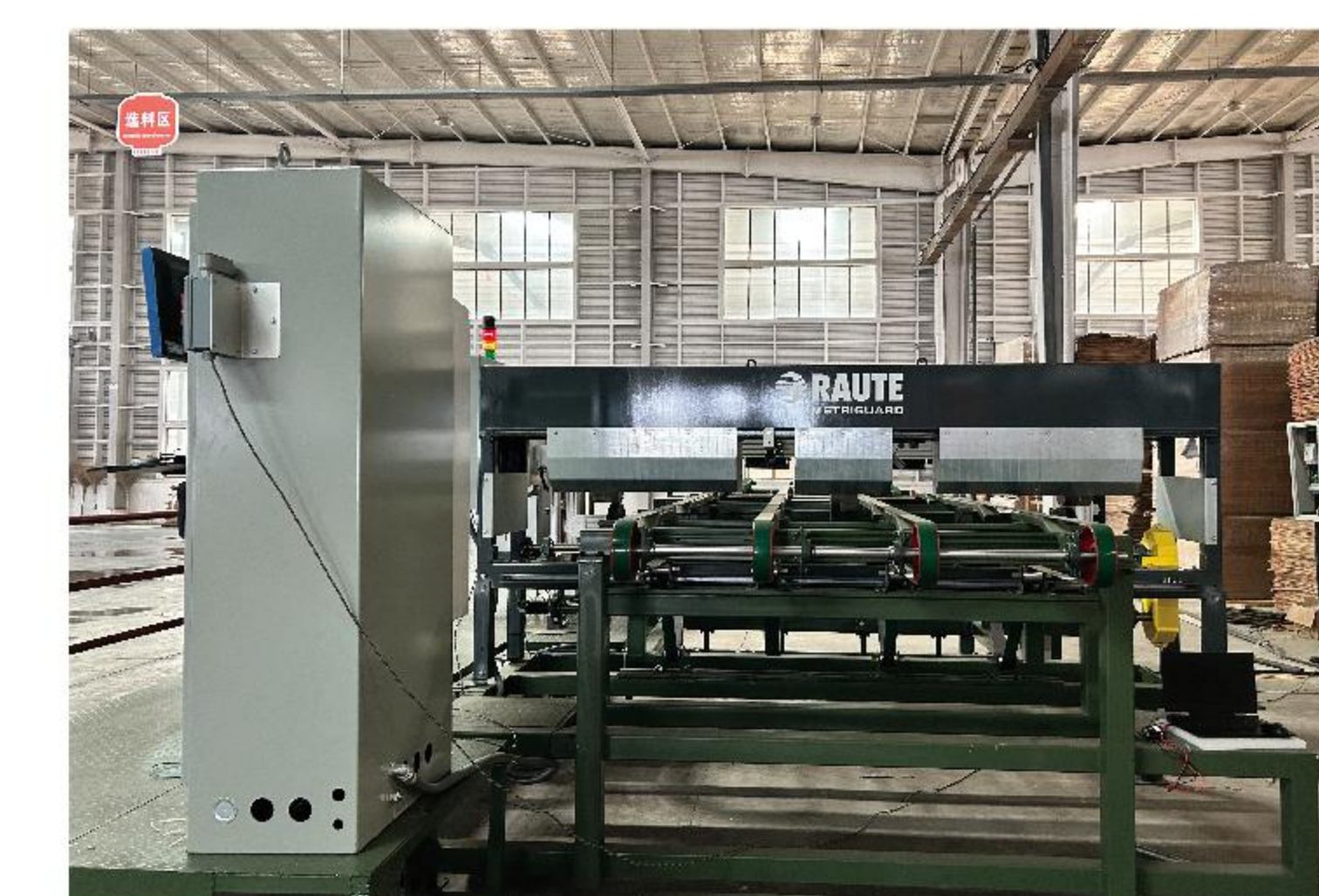
单板分选机 Veneer grading system
